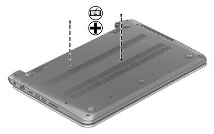
2. Turn the computer right-side up with the front toward you. Open the display and stand the computer on its right side. Insert a thin tool through the keyboard access hole. (The keyboard icon indicates the keyboard access hole.) Push firmly on the bottom of the keyboard until it disengages from the computer.
